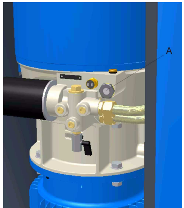
Fig. 9.1 - Oil Level Sight Glass Location
